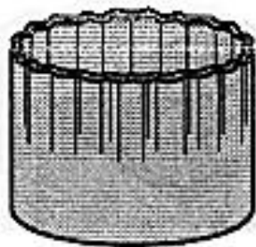
(b) Wrinkling in the wall
